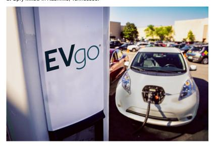
The completed station at 433 Opry Mills Drive includes two (2) 480V Fast Chargers manufactured by BTC Power. Each one can deliver a 50 kilowatt charge at the same time, which provides 80% State of Charge in 30 minutes, or about 150 miles of range per hour.
